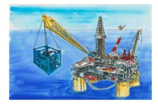
A crane was used to support 3" polyurethane hose to a height of 165'. The vacuum system raised the debris to the 165', and then pulled it down through 4" hose to the Collection Tank. Additional lifts through the tankage system made the total lift close to 200' (60 m). A recovery rate of 6000 lbs/hr was achieved during the demo. No additional air supply was needed.
