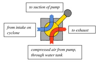
Pressure Mode (valve handle in horizontal position; shown slightly off for clarity):
