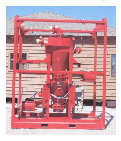
Product is loaded in the top via 6" intake line (vacuum connects to the 4" fitting at very top). There are two 12" knife valves. The center knife valve automatically opens on timed relay (generally 20-30 seconds) when the top hopper is full, dumping contents to the bottom hopper. That valve closes, and refilling of the top hopper resumes. The bottom knife valve dumps to an auger for conveyance. In that manner, vacuum is never lost.
