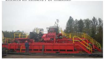
Halliburton Baroid's Two-Stage Hammermill unit
