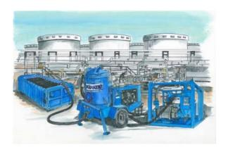
Triton's 500 Series Trailer mount vacuum unit proved to be a cost effective answer to this challenge. The 500 Series vacuum unit consists of a trailer mount 500 cfm vacuum pump with a 10 bbl tank allowing you to pull and discharge the water and sludge without the need for additional equipment.
