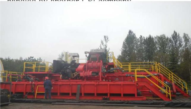
*Halliburton Baroid's Two-Stage Hammermill unit*
